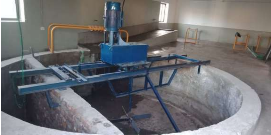
Picture 1: Collection Hall, Cow stomach cleaning area, Slurry Mixing Tank and Mixing Machine
